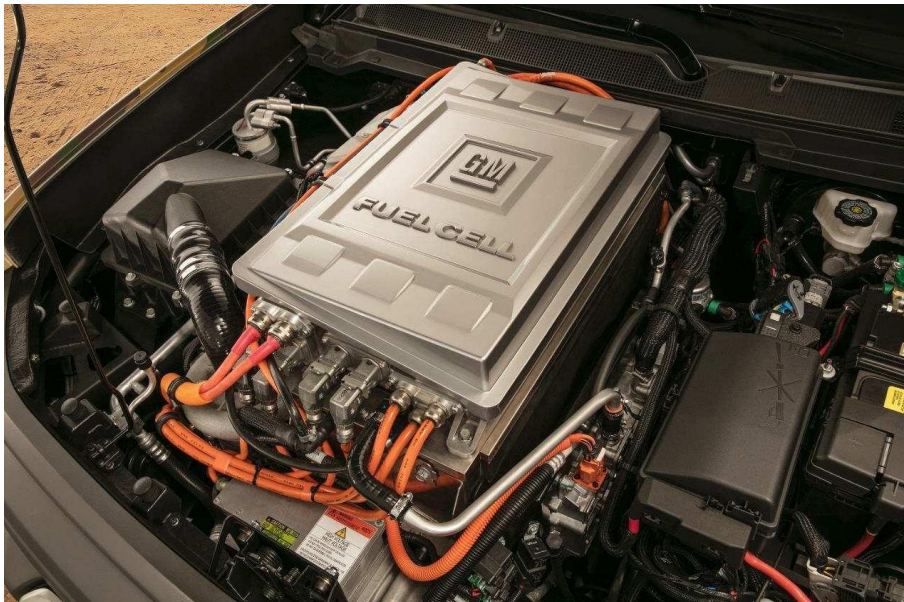
Figure 18 - La pile de la Colorado ZH2
